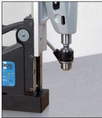
2. Place drill chuck in MT arbor.
