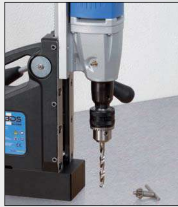
3. Ready for use with twist drill.
