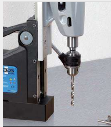
3. Ready for use with twist drill.
