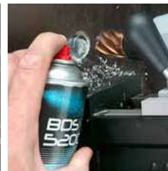
Step 2: During drilling, spray the high-performance lubrication spray onto the tip of the drill and into the cut hole.
