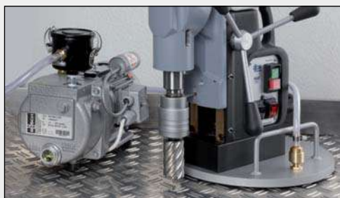
ZAV 300 Vacuum clamping device for channelled and gusset plates
