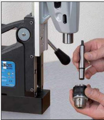
1. Connect taper drift to drill chuck.
