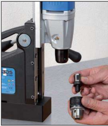
1. Connect adapter to drill chuck.
