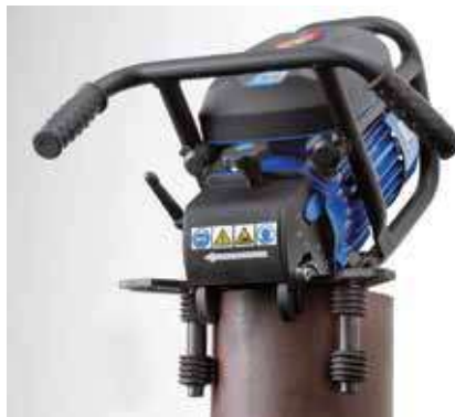
Edge machining on vertical pipes
