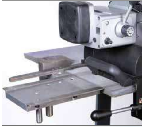
Inlet/outlet rails of the AutoCUT 500
